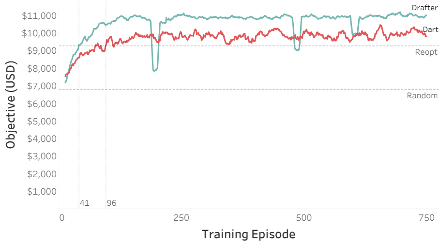
Figure 5: Training curves for the Dart and Drafter agents, showing two-week performance averages (the average objective over an episode and the previous 13 episodes). Dashed horizontal lines depict mean objective values for the Random and Reopt agents. Vertical lines indicate where Dart and Drafter surpass Reopt’s mean objective achievement.
